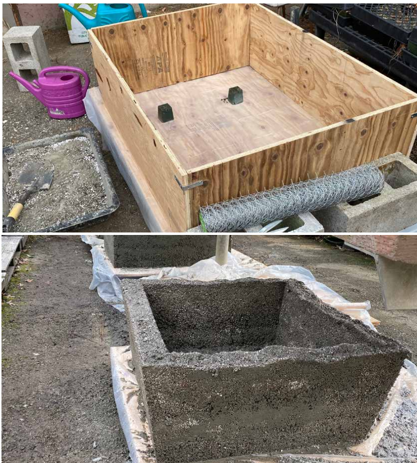
Wooden mold for trough construction (top) and a finished trough (bottom)
