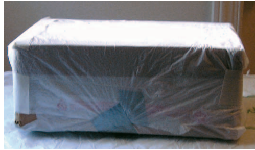
PROJECT B: Cardboard box ready to be used as trough form. Stuffed with paper, wrapped in plastic, ready for an outer layer of papercrete an inch or more thick. Feet will be added on top. After papercrete hardens, turn trough right side up, slit visible plastic and underlying cardboard, remove stuffing. Pull box from trough.
